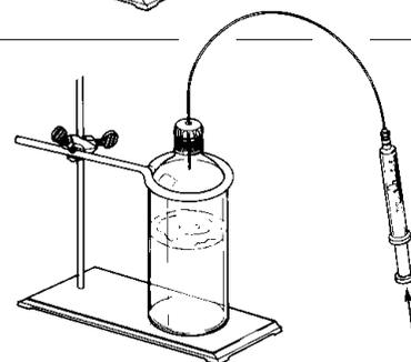
Fig. 10. Syringe transfer of reagent to reaction vessel
