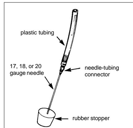
Fig. 2. Nitrogen-flushing needle
