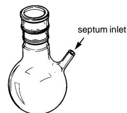
Fig. 4. Flask with septum inlet
