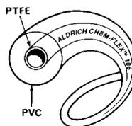
Developed by Aldrich for the safe transfer of aggressive solvents, air-sensitive liquids and gases. Chemflex is constructed of a thin inner-tube of PTFE sheathed in clear PVC. CHEM-FLEX 106 tubing designed specifically for use with 12 gauge transfer needles and is suitable for small volume transfers of products packed in Aldrich Sure/Seal bottles.
