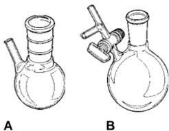
A. Round bottom flask with ground-glass joint and septum inlet.
