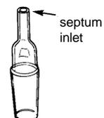
Fig. 5. Septum inlet adapter
